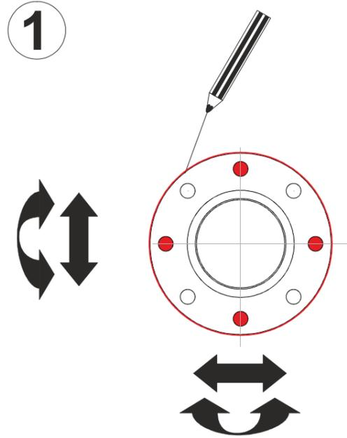
**1** Determine the position of the product. Mark the outline and position of the holes on the sub-soil.
