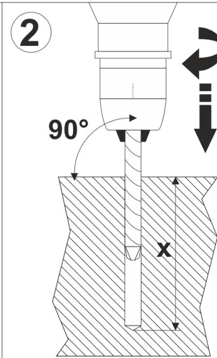
**2** Drill holes in the sub-soil using the concrete drill Ø 10 mm. Depth as shown in the products drawing.
