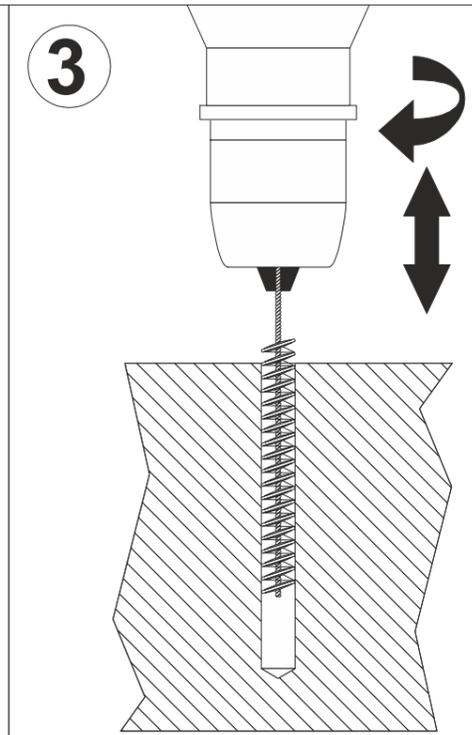
**3** Brush the holes using the steel brush (Ø 11 mm). Clean the holes.
