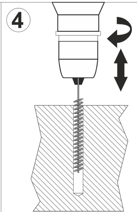
Brush the holes with the steel brush (Ø 11 mm). Remove any dust.
