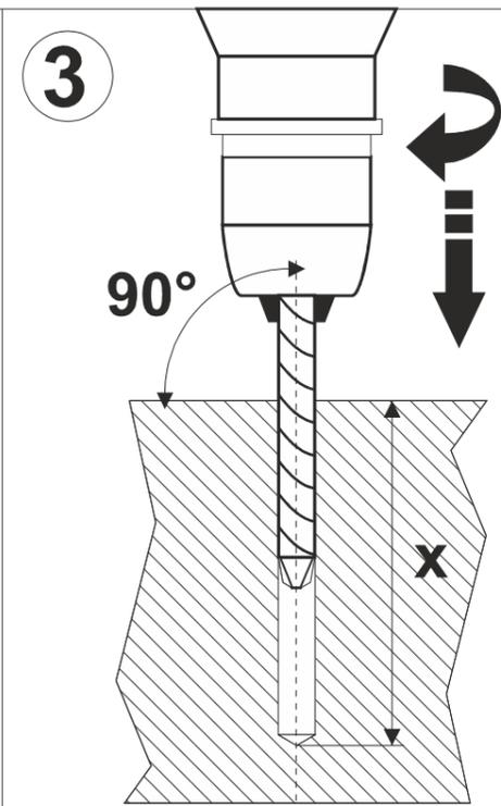
Drill holes Ø 10 in the sub-soil. Drilling depth is shown in the attached drawing.
