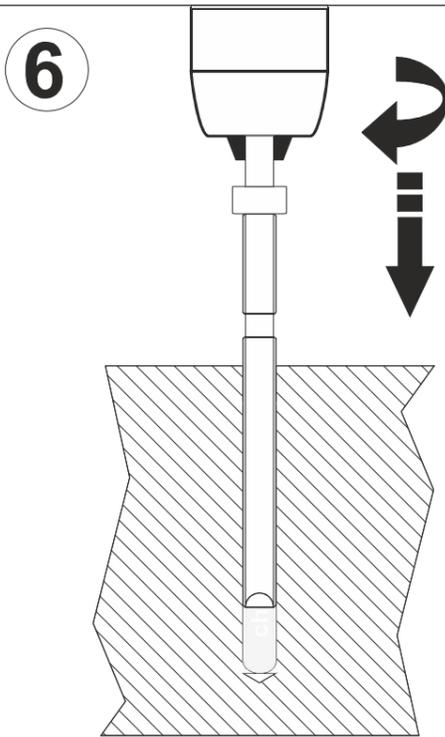
Insert anchor shaft, using the delivered tool.
