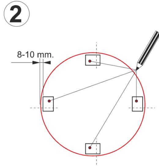
Position the PVC blocks at a distance of 8-10 mm from the edge of the product (as shown in drawing 2.3.1)
