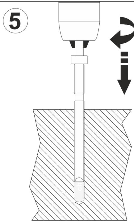
**5** Place anchor shaft using the delivered tool.
