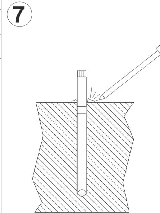
**7** Remove any remains around the anchor shaft.
