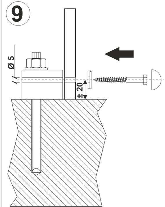
Place the product over the blocks. Drill a hole Ø 5 mm through the product in each of the PVC blocks. Fix the product on the blocks with the bolts Ø 6x50 mm. Put a nylon cap on every bolt.
